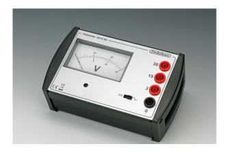
The voltmeter 3815.60 is a sturdy instrument for both AC and DC which is specifically designed for use by students. The instrument is provided with a DC/AC switch and three voltage ranges.
