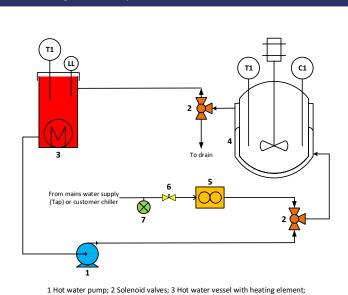
4 Crystallisation vessel; 5 Flowmeter; 6 Needle valve; 7 Pressure regulator
