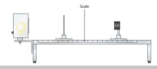
Schematic diagram showing HT13 set up for exercises using light
