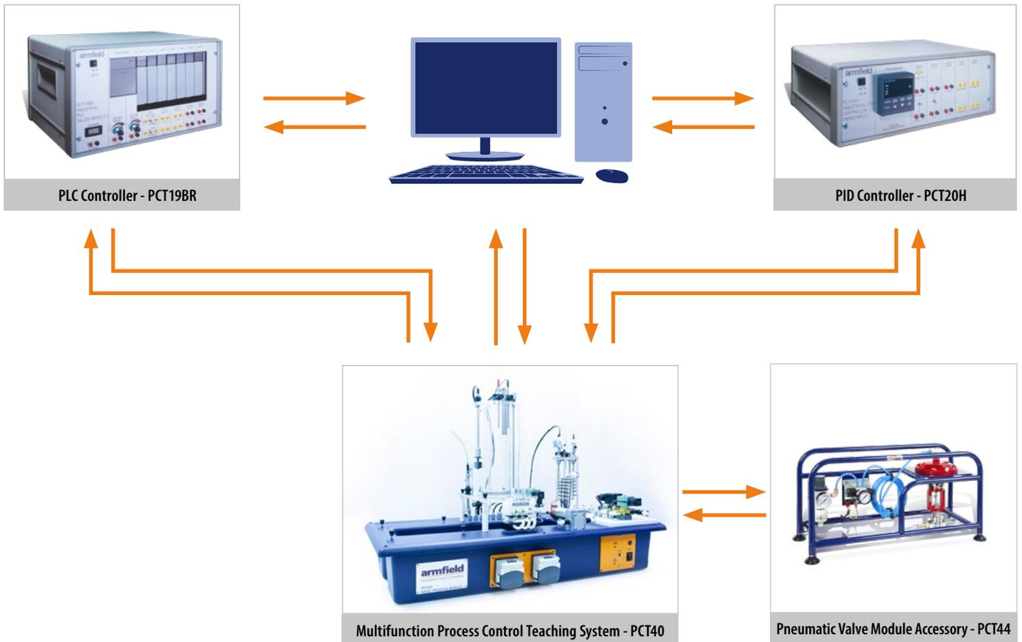
It is possible to control the PCT40/41 loops using external PLC devices or PID controllers. These can be connected directly to the PCT40 for specific configurations. However, with the PCT43 electronic console it becomes very easy to connect up the inputs and outputs to enable a range of loops to be demonstrated.
