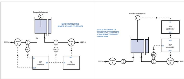
Fig 1: Ratio control of two flows
