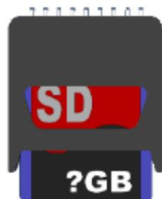
The SD card component can be used to enhance storage capacity of the MIAC when used in conjunction with an optional micro SD card inserted into the internal micro SD card slot.
