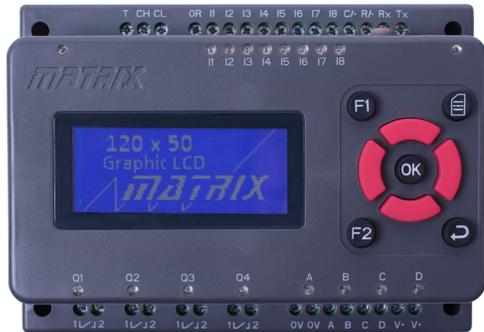
The MI5769 and MI6693 MIAC versions have a 4Gb Compute module that is pre-loaded with the Raspbian operating system, including Python and Node-RED. Additionally, MIAC specific kernel drivers are pre-installed.
