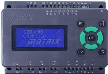
MI5331 AllCode dsPIC33EP256MU806 16 bit processor module
