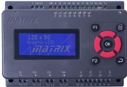
MI5769 Raspberry Pi compute processor module
