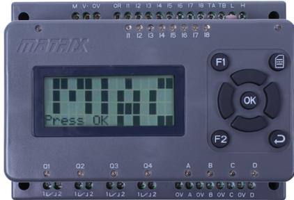
MI0235 PIC PIC18F4550 processor module
