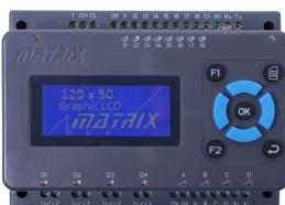
To deploy your project to the PIC and dsPIC versions of MIAC, connect via USB cable and power the MIAC.
