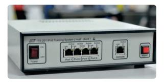
ITS-201 (host : client) can simulate over 10 kinds of packet protocols. It supports IPv4 and IPv6 Dual-Stack system and Remote Packet Capture Service (RPCAP). Using filterable TAP configure load-balancing and port-bonding to avoid browsed packet loss.
