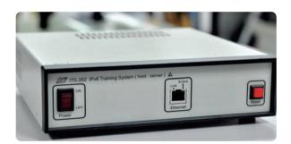
ITS-202 (host : server) is designed by a series of internet service and web-based GUI interface. ITS-202 can be easily configured as 5 types of servers to observe the behaviors in real applications behavior.
