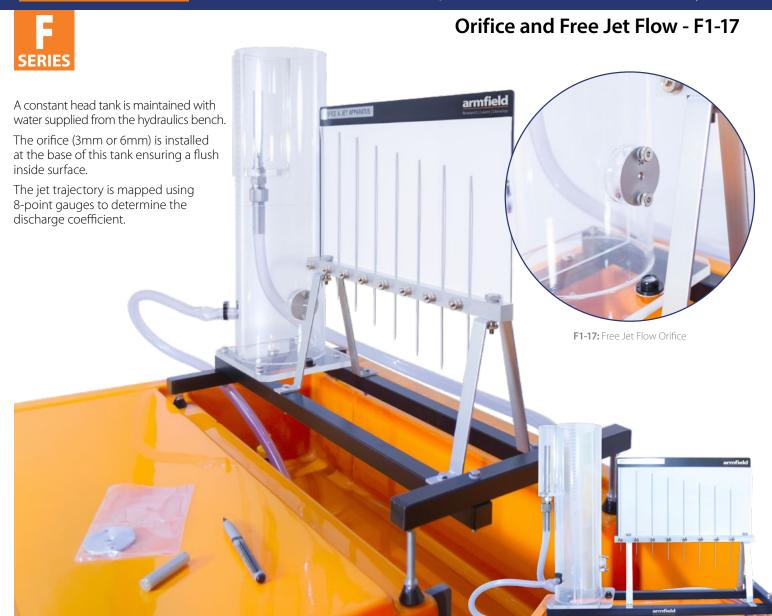
This equipment permits calibration of two orifices of differing diameter and enables the trajectory of the jet to be plotted.
