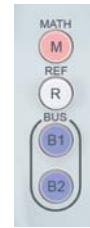
The GDS-3000 Series provides two dedicated keys in the front panel for two sets of setting recall
