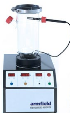
FT31 with 5l tub with bag and temp humidity probe
