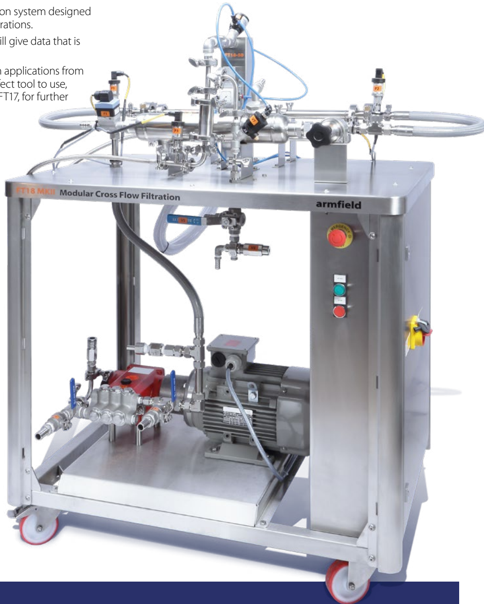
FT18-MkII-50-1 shown with Backpulsing/Backflushing options FT18-5 Ceramic Filter Module fitted. Bellow touch screen (option)
