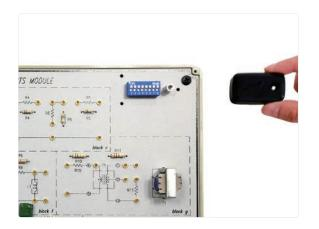
Each module is equipped with an 8-bit DIP switch for fault simulations. Users can practice trouble shooting by setting the DIP switch to different positions.
