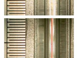
Images show how the level of acetone in the capillary tube falls over time, and how the software accurately measures the level
