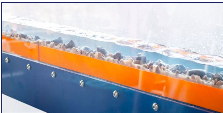
C4-69 - Artificially roughened bed
