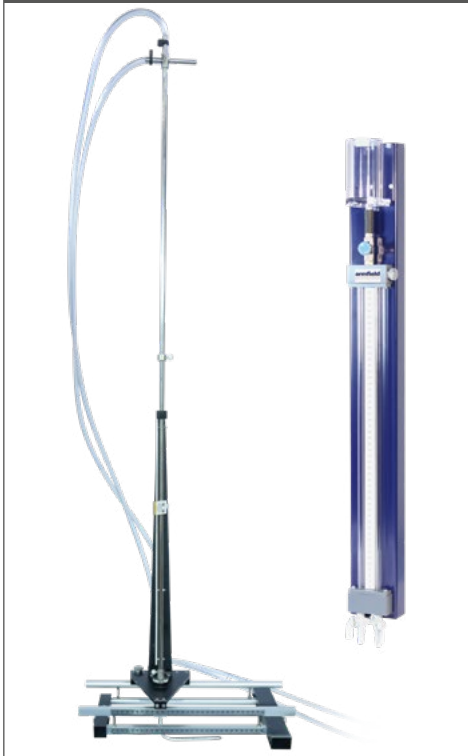
C4-61 - Pitot tube and manometer
