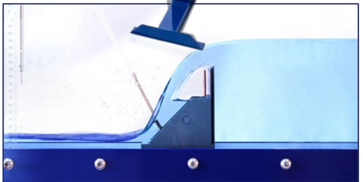
Sharp Crested Weir (in vented condition)
