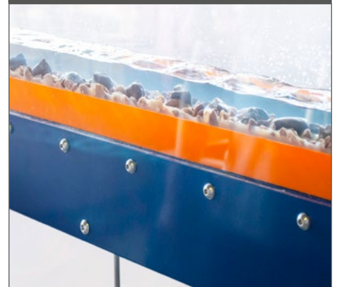
C4-69 - Artificially roughened bed
