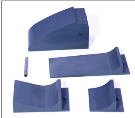
C4-64 - Free overflow spillway section complete with ski jump, sloping apron and blended reverse curvature attachments
