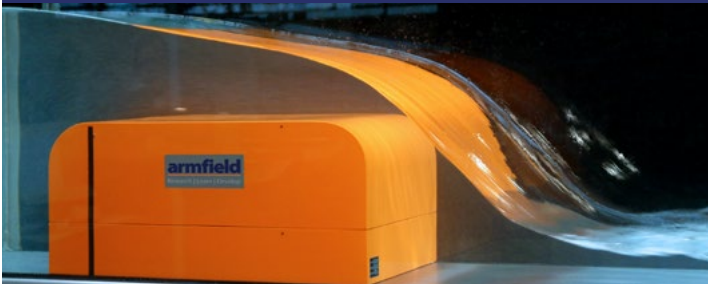
S6-23: Ogee Weir & Manometer Board
