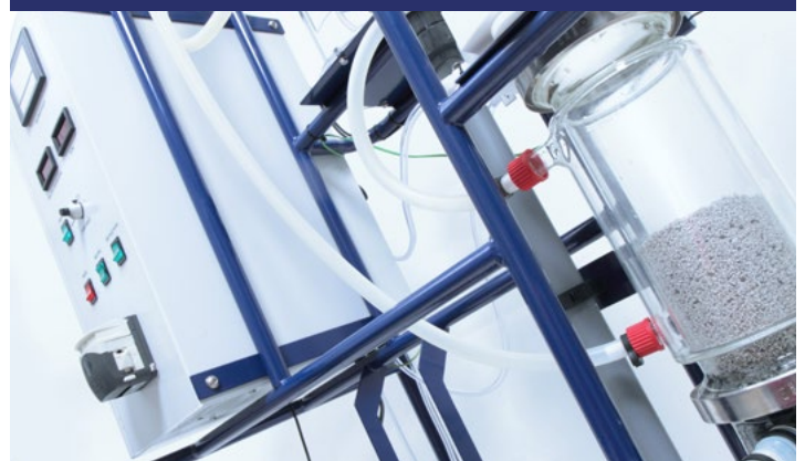
Control cabinet and pumice bed material in heated jacketed vessel
